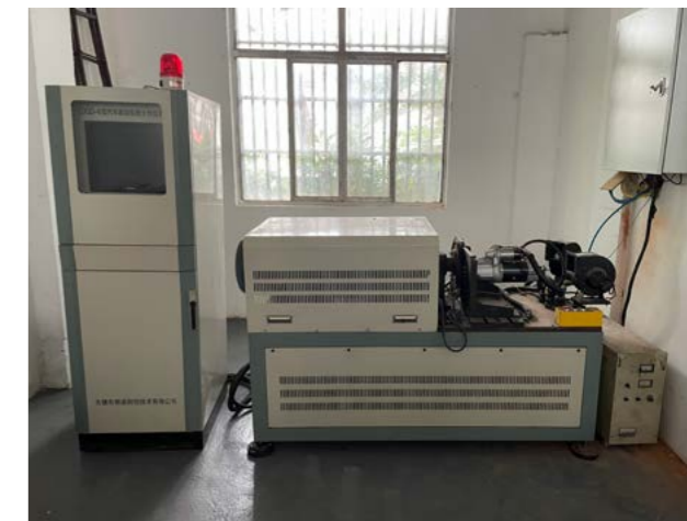
Starter endurance test bench
